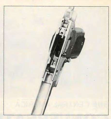
ABOVE: Investment-cast frame of S&W M645. BELOW LEFT: Field-stripped S&W M645. BELOW RIGHT: Good feed angle assures reliable feed.
